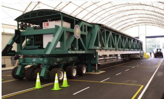
Airport Pavement Test Facility (NAPTF) Heavy Vehicle Simulator, Mark VI (HVS)
